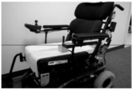
Butt Scooter mounted on powered wheelchair. Conveyor fabric on cushion
