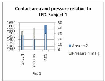
(yellow LED), properly inflated (green LED) and underinflated (red LED) cushion. Figures 1-3 indicate the expected relationship between contact area and pressure. We observed the lowest interface pressures with the red LED illuminated in all of the trial measurements (10 total). The highest interface pressure related inversely to the lowest contact area. These values were intermediate when the green LED illuminated.
