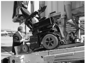
Device to block wheelchairs from tipping backward when placed on the conveyor belt (Photos courtesy of Eric Lipp, Open Doors Organization).
